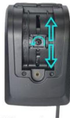
3. Unscrew the screw and adjust the lens
