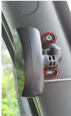
4. Adjust the left and right angle joints of the DMS camera through the hexagon socket screws, so as to adjust the angle of the DMS camera left and right.
