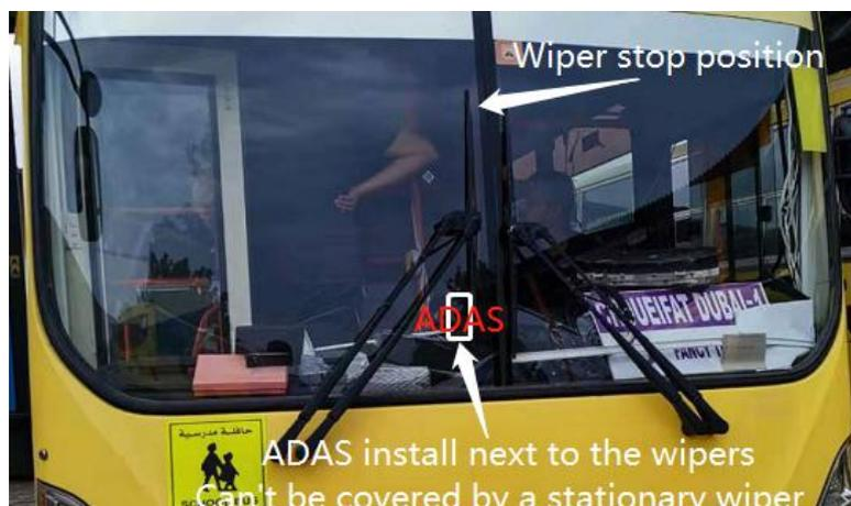
4. Make sure that ADAS is installed within the working area of the left and right windshield wipers (so as to ensure that the area within the range of the ADAS camera lens can be cleaned by the windshield wiper).
