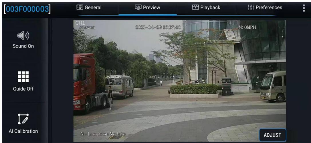
Enter the real-time preview interface and double-click the ADAS channel screen to enter the main stream, and then click "AI Calibration" at the lower left corner of the screen to enter the AI calibration selection interface for ADAS calibration.
