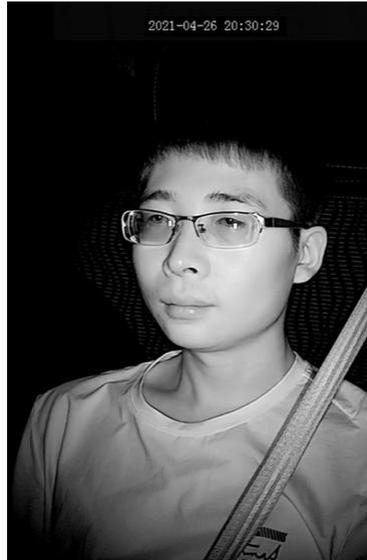
2. Make sure that the fill light of the DMS camera faces towards the driver's face (the fill light shall not face towards the seat belt; otherwise, it will lead to overexposure of video).
