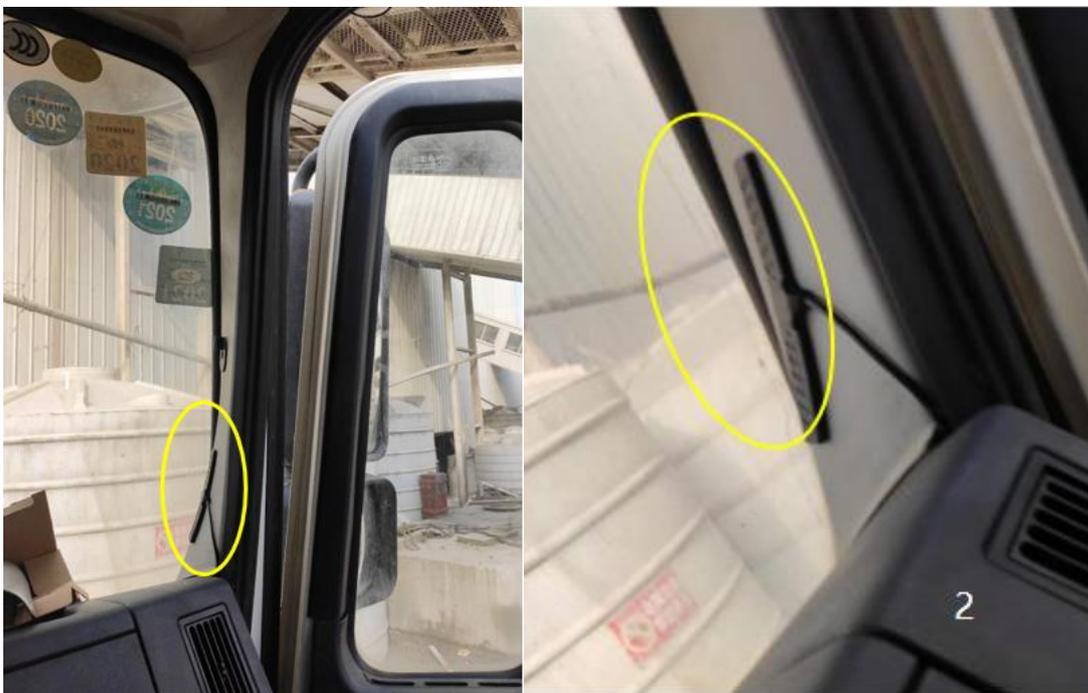
Tear off the 3M adhesive film on the 3G/4G antenna and stick the antenna under the A-pillar at the front passenger side.
