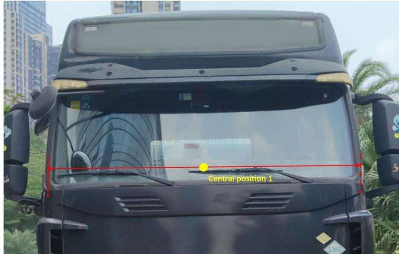
Next, in the vertical direction, locate another horizontal center point 2 on the front windshield at least 20 cm away from center point 1. Connect center points 1 and 2 with a mark pen, to draw the centerline of the front windshield.
