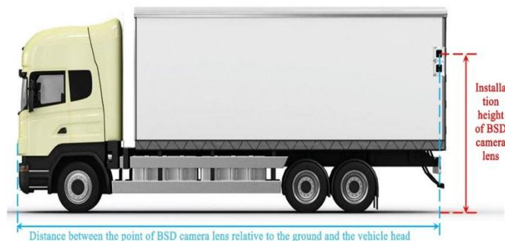
2. Click "Setup - Basic Setup - Other Setup – Algorithm – BSD Install Height" in sequence, and then enter the following two values: distance between the point of the BSD camera lens relative to the ground and the vehicle head, and installation height of BSD camera.
