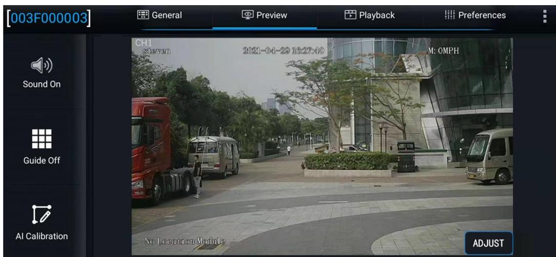
Enter the real-time preview interface and double-click the ADAS channel screen to enter the main stream, and then click "AI Calibration" at the lower left corner of the screen to enter the AI calibration selection interface for ADAS calibration.
