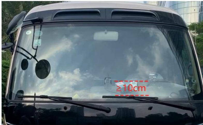
3. If the wiper stops vertically in the middle of the front windshield, the ADAS camera lens shall be installed as close to the middle position as possible (to avoid too high sensitivity for any lane deviation on this side) and be less than 10 cm away from the centerline, provided that the lens will not be covered by the windshield wiper at stop position.
